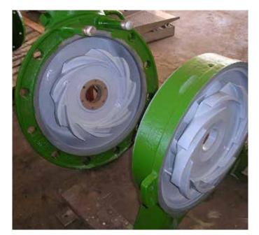
Belzona 1341 (Supermetalglide) is a two-component coating system designed to improve the efficiency of fluid handling equipment and to protect metals from the effects of erosion-corrosion.
